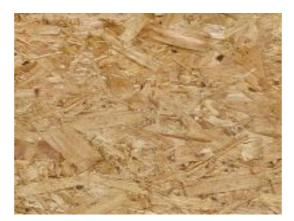
The desk itself is made from chipboard otherwise known as particleboard; this unusual material is low cost and can be highly sustainable when manufactured correctly.
